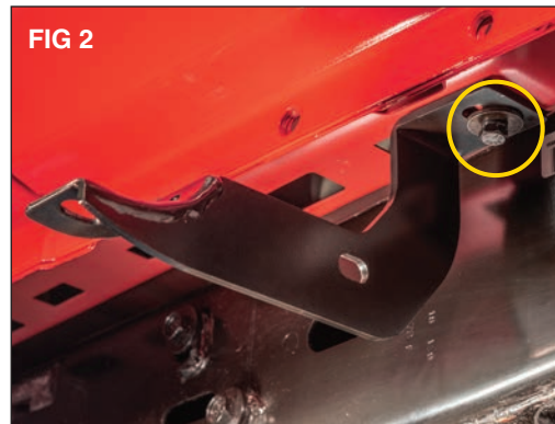
FIG 2 Align the hole in the step mounting bracket (PF) and loosely install using a 8 x 35mm bolt (B), lock washer (J) and flat washer (H). (FIG 2)
