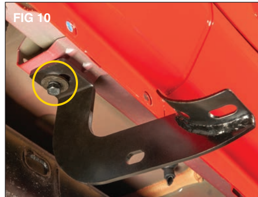
Align the hole in the step mounting bracket (PR) and loosely install using a 8 x 35mm bolt (B), lock washer (J) and flat washer (H). (FIG 10)
