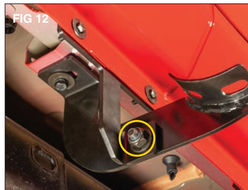
Next align the mounting slots between the two brackets and loosely install a 10mm bolt (A) with washers (G) on both sides and secure with a 10mm nylock nut (E) using a 16mm hex wrench and a 17mm socket. (FIG 12)
