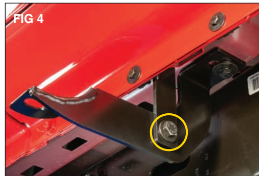
FIG 4 Next align the mounting slots between the two brackets and loosely install a 10mm bolt (A) with washers (G) on both sides and secure with a 10mm nylock nut (E) using a 16mm hex wrench and a 17mm socket. (FIG 4)
