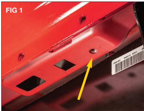
FIG 1 Put on safety glasses. Starting at the front of vehicle locate the vertical threaded hole behind the pinch weld. (FIG 1)
