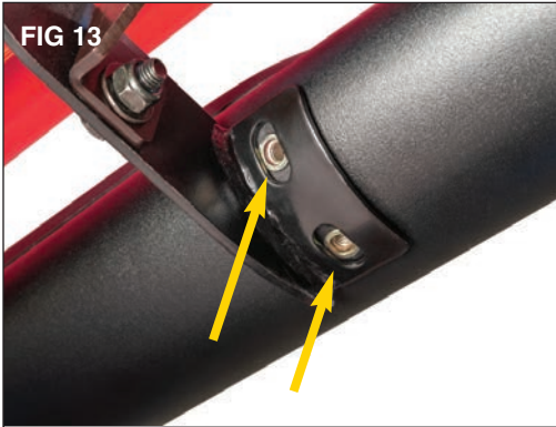
Now align the step with mounting bracket holes as shown. (FIG 13)
