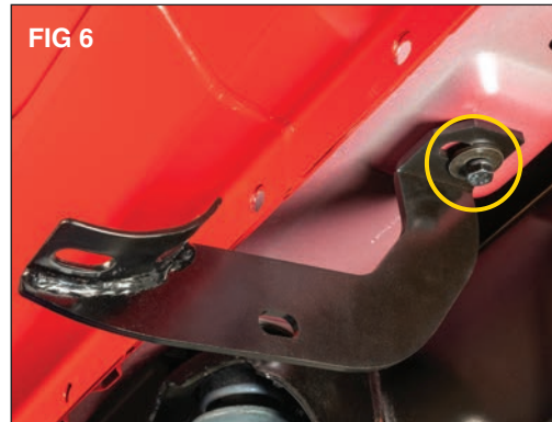
Align the hole in the step mounting bracket (PM) and loosely install using a 8 x 35mm bolt (B), lock washer (J) and flat washer (H). (FIG 6)
