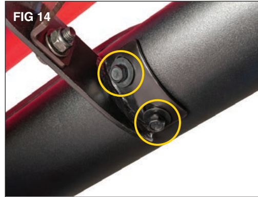
Loosely install the 8mm bolt with captive washer (D) using a 13mm socket. (FIG 14)
