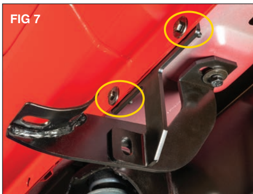
Locate and loosely install the center support bracket using 6mm hex head bolts (B) through the pinch weld with washers (I) on both sides and secure with a 6mm nylock nut (F) using a 10mm hex wrench and a 10mm socket. (FIG 7)
