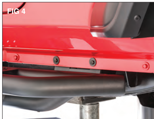
Do not fully tighten at this time. Repeat on the 3 remaining holes. (FIG 4)
