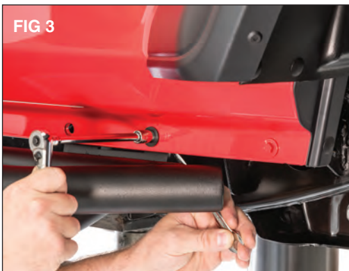
Install the 6mm hex head bolts through the pinch weld and the mounting bracket with washers on both sides and secure with a 6mm nylock nut using a 10mm hex wrench and a 10mm socket. (FIG 3)
