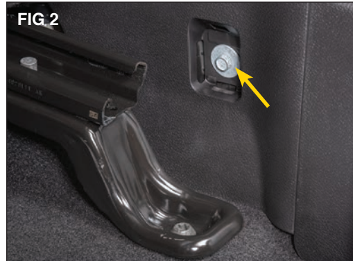
tool. (FIG 1) Remove both bolts using a 10mm socket. (FIG 2)
