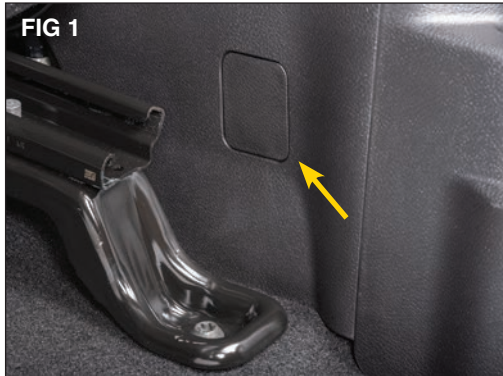
Put on safety glasses. Slide both seats forward. Locate both of the trim panel covers and remove using a trim removal
