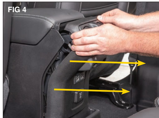
Carefully pull backward on the center console vent panel to release the clips. (FIG 4)
