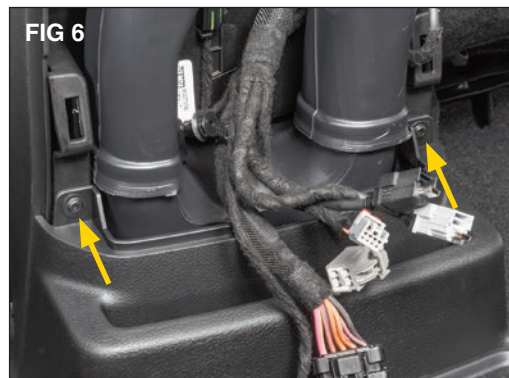
Remove the two screws at the top of lower tray using a T-20 torx driver. (FIG 6)
