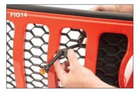
Slide the light mounts over the wire loom as shown. (FIG 14) Snap each diamond-shaped light mount into the the correct grill. Squeeze the bottom
