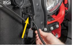
Fish it through the rubber barrier on the driver side of the radiator as shown.
