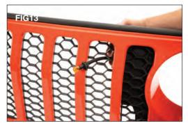
front camera you will need to lower the light in the center slot and the other two to match if desired. Next, carefully separate the rubber grommet from the light and fish them through each hole in the grill to be used. (FIG 13)
