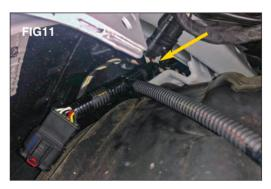
the OEM harness until you hear a click and then push the red and gray locking tabs to lock the connections. (FIG 11)
