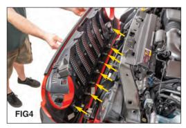
Gently tilt the grille forward and then gently pop the lower portion of grille from its (8) retaining clips. (FIG 4).
