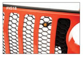
Push the LED light into the rubber grommet to seat the light into the mounting bracket. (FIG 18)
