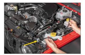
Route the harness behind the headlight and past the reservoir bottle towards the firewall on the divers side.
