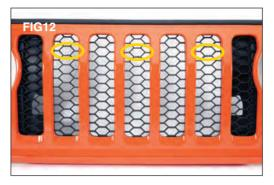
With the wiring now routed towards the grill, Locate the 2nd, 4th and 6th slots in the grill as shown (FIG 12) Then locate the 2nd from the top complete diamond shape, this is where to place the lights. Note: On models with the
