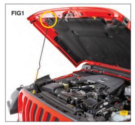
Put on safety glasses. Open the hood of your Jeep<sup>®</sup>. Put the prop rod into the correct slot to hold hood open (FIG 1).
