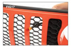
Slide the rubber grommet down the loom and push it into the light mount. (FIG 17)
