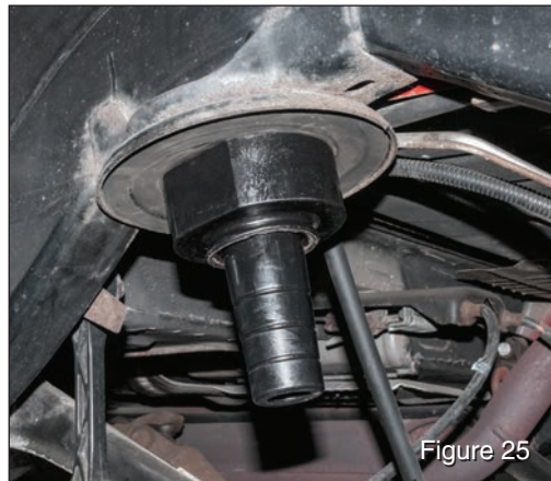
While holding the coil spacer in place, Re-attach original bump stop assembly using the original bolt, 15mm socket with ratchet extension and tighten. (FIG 25)
