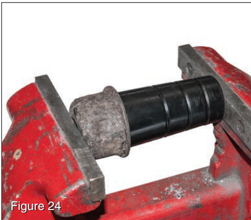
Lubricate the provided bump stop with dish soap and press it into the original bump stop cup. We found it easier to use a vice. (FIG 24).
