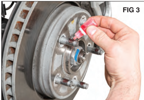
Apply the provided thread locker to the original wheel studs as shown. (FIG3)
