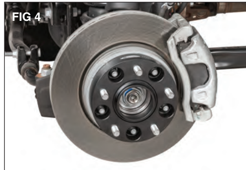
Slide wheel spacer and or adapter on to wheel studs as shown. (FIG4)
