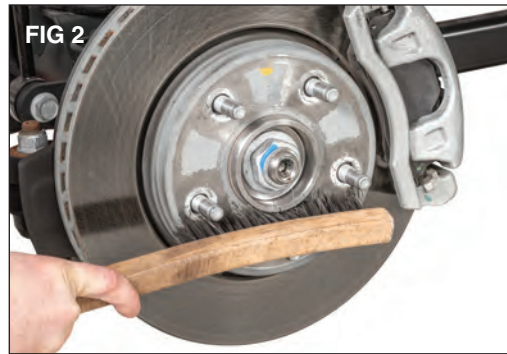
Thoroughly clean wheel studs, hub area, brake drum and or rotor disc using a wire brush. (FIG2)
