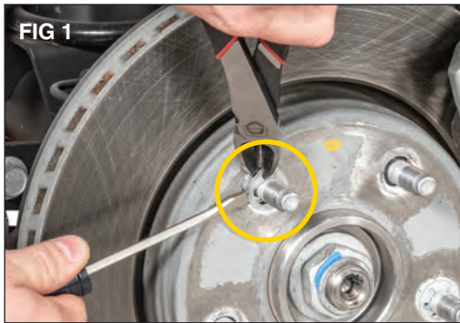
If present, remove brake drum or rotor disc retaining clips using a flat blade screwdriver & diagonal pliers. (FIG1)
