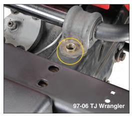
For use with a stock TJ bumper, place the supplied spacer rings over the sway bar bolt holes on both sides.
