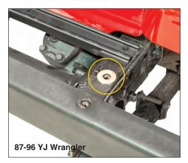
When installing winch plate on a YJ with a stock bumper place a supplied ½" washer over second bumper hole.
