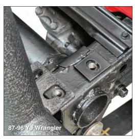
If you are installing the winch plate on a YJ Wrangler with a Tube style bumper place the supplied spacer plates over the 2nd mounting holes in your frame as shown above. Repeat for other side.
