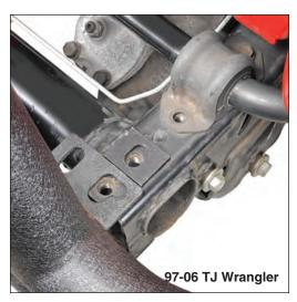
If you are Installing this winch plate on a TJ Wrangler with a tubular bumper use the supplied spacer plates under the 2nd bumper bolt hole in your frame as shown above.
