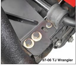
For either a stock or tubular bumper: For TJ, Position winch plate so that it is aligned over the 3 mounting holes per side. Install the supplied 10mm x 50mm sway bar bolts with a lock washer & flat washer using a 16mm socket. Then install supplied 1/2" bolts with a lock washer & flat washer using a ¾" socket, as shown above.
