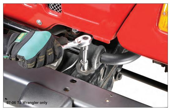
For 97-06 TJ Wrangler only: Remove the 2 front sway bar retaining bolts with a 15mm socket. Do not remove the rear swaybar mounting bolts.
