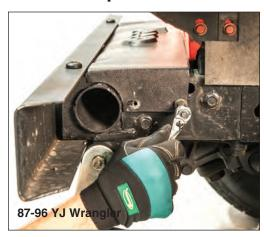
Put on safety glasses. Remove frame / sway bar cover by removing the 2 bolts on either side with a 3/8" socket.
