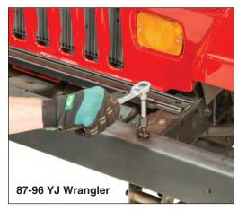
Remove the upper bumper bolts using a T55 Torx bit. (2 on YJ / 4 on TJ) Do not remove the lower bumper bolts.
