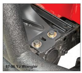
For either a stock or tubular bumper: for YJ, align the winch plate over the two correct holes, install the supplied 1/2" bolts with a lock washer and a flat washer and tighten using a ¾" socket.
