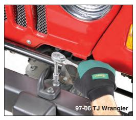
If your vehicle is equipped with Tow hooks retain the bolts and tow hooks for reassembly.
