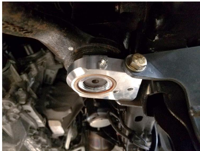
Figure 16. Installing Hardware in Synergy Sector Shaft Brace
