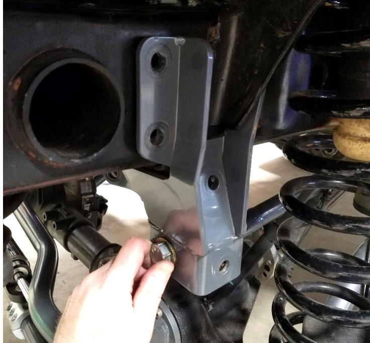
Figure 7. Synergy Track Bar Brace Loosely Installed
