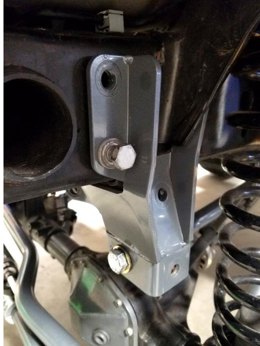
Figure 8. Threading Bolts into Steering Box
