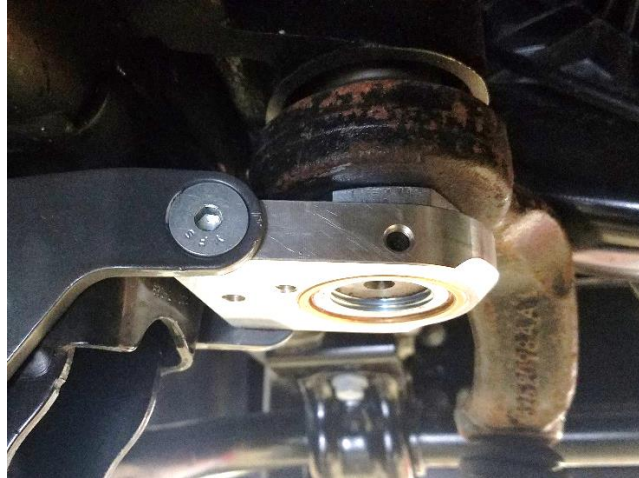
Figure 17. Installing Flat Head Screw in Back of Synergy Sector Shaft Brace
