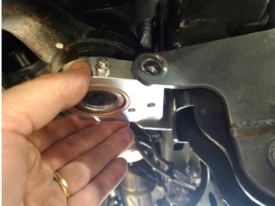
Figure 15. Installing Synergy Sector Shaft Brace on Pitman Arm Nut
