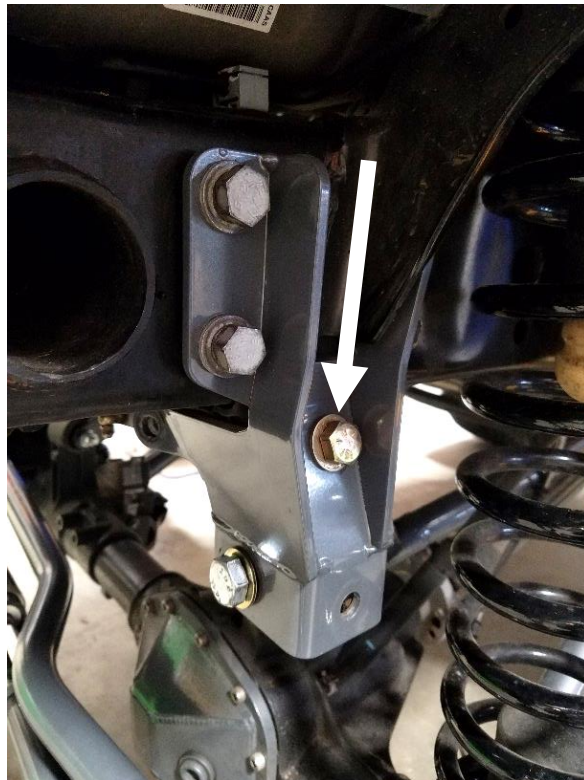
Figure 9. Installing Upper Track Bar Mount Hardware
