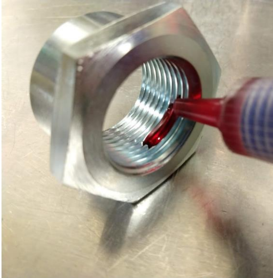
Figure 4. Adding Threadlocker to Nut
