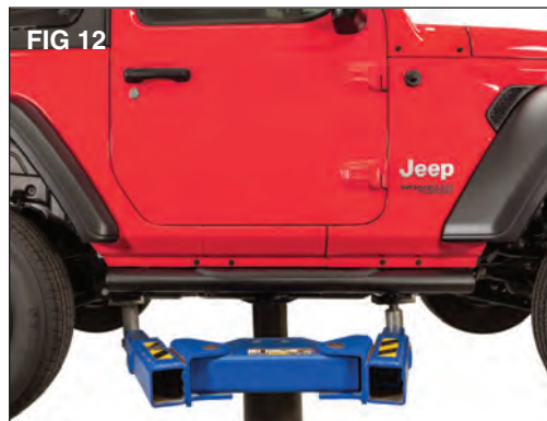
Now tighten the 10mm hardware securing the brackets to each other. Lastly tighten the 8mm captive washer bolts to tube step. Each bolt is tightened to the Torque Specs show below.
