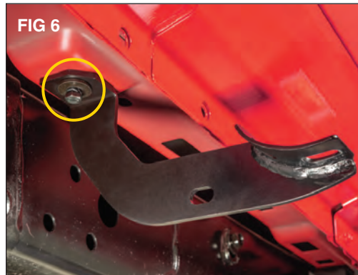
Align the hole in the step mounting bracket (PC) and loosely install using a 8 x 35mm bolt (B), lock washer (J) and flat washer (H). (FIG 6)
