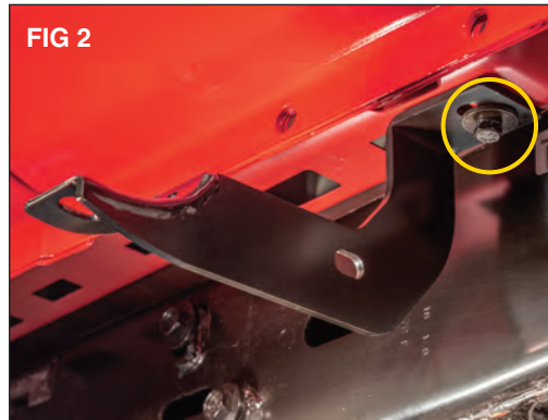
Align the hole in the step mounting bracket (PF) and loosely install using a 8 x 35mm bolt (B), lock washer (J) and flat washer (H). (FIG 2)
