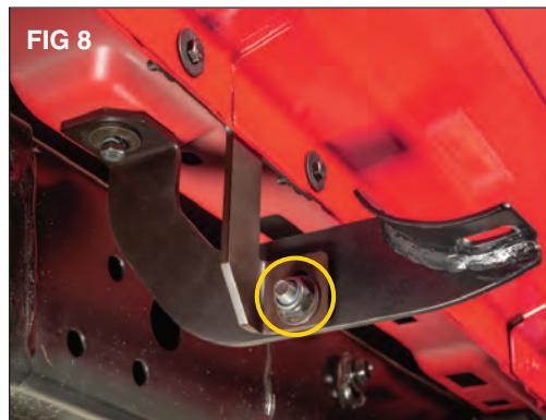
Next align the mounting slots between the two brackets and loosely install a 10mm bolt (A) with washers (G) on both sides and secure with a 10mm nylock nut (E) using a 16mm hex wrench and a 17mm socket. (FIG 8)
