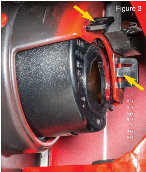
With the bulb and socket removed, locate the two housing retaining tabs (Fig 3) and gently pry with a small flat-blade screwdriver outwards to release
