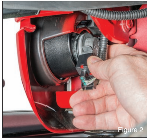
Remove the bulb and socket assembly from the housing by twisting the socket down towards the ground one quarter of a turn until it loosens (Fig 2).
